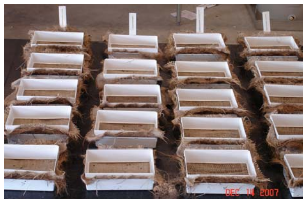
Fig.4. Lab bioassay conducted once every two weeks during a 9-month aging period to evaluate the efficacy of bifenthrin-treated burlap on fire ant female alates.
