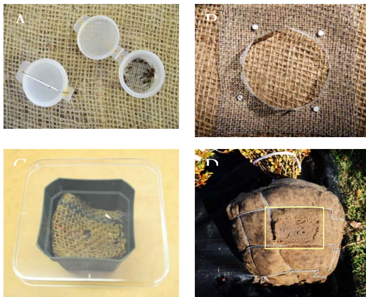
Fig 2. A): Small basket with a wire-meshed bottom allowing alates to contact with the treated burlap underneath for bioassay conducted directly on rootballs. B): wire mesh cage attached directly onto rootballs (without showing the snugly fit Petri dish cover). C): Method of choice-- apparatus for bioassay conducted in the lab. D): rootball showing a piece of burlap was removed for bioassay in the lab; soil sample was also collected from where burlap was cut out (within yellow rectangle).
