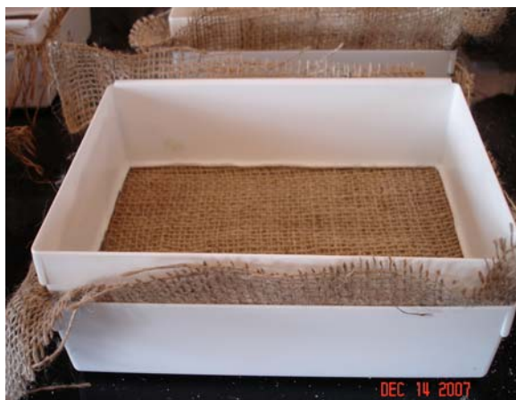
Fig.1. One treatment unit setup: a layer of bifenthrin-treated burlap secured in between two plastic boxes with the top box's bottom cut out and wall coated
