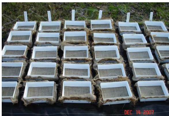
Fig.3. Treatment units with bifenthrin-treated wrapping materials aging outdoors with exposure to sunlight, rain, and daily irrigation simulating nursery storage
