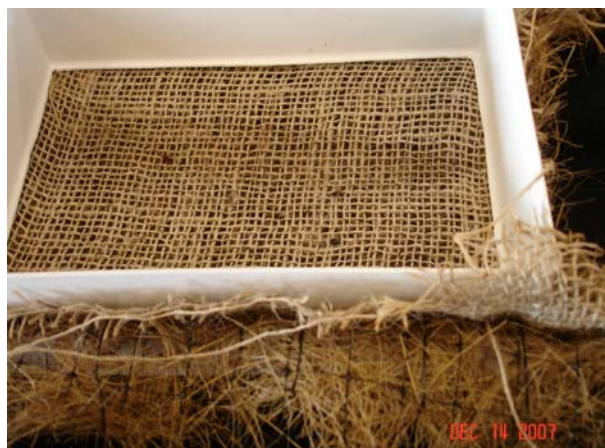
Fig.2. Similar treatment unit showing an extra layer of coconut blanket attached under the burlap layer. Only one layer of the wrapping materials was treated with bifenthrin when more than one layer was
