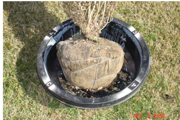
Fig.10. Intact root ball bioassay: This method is an outdoor version of the lab bioassay on treated burlap. Using a real root ball to test it outdoor will be closer to reality.
