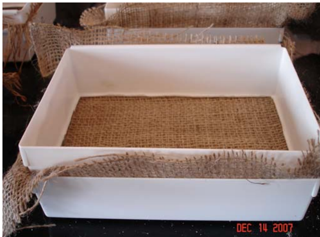
Fig.1. One treatment unit setup: a layer of bifenthrin - treated burlap secured in between two plastic boxes with the top box's bottom cut out and wall coated with Fluon.
