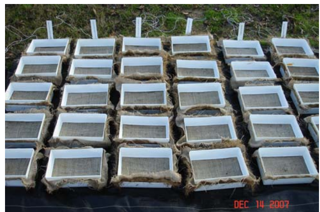
Fig.4. Treatment units with bifenthrin-treated wrapping materials aging outdoor for exposure to sunlight, rain, and daily irrigation.
